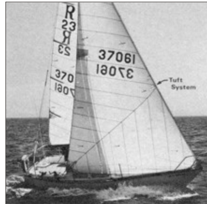
Figure 1. Mainsail and genoa set up for telltales and tufts.
