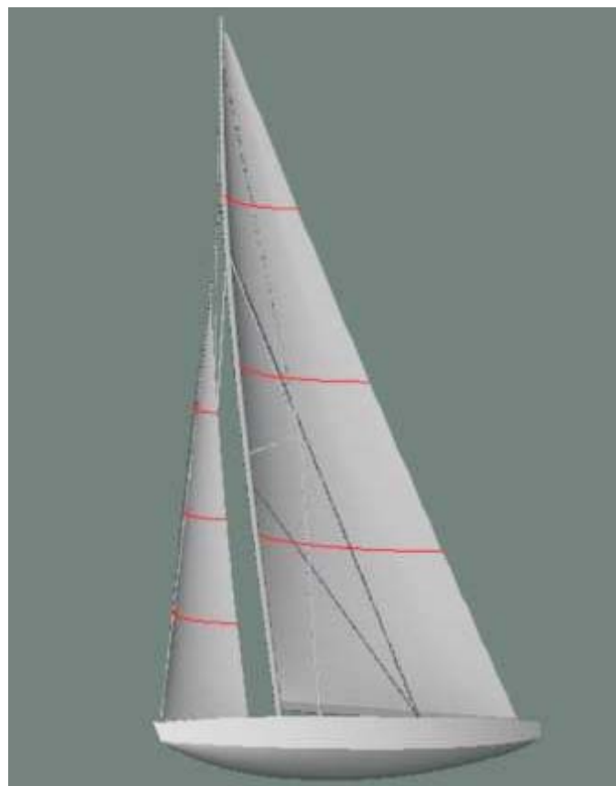
The Star as represented in the Boeing Aero Grid and Paneling System.
